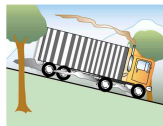
Figure 14.5 The smoking brakes on this truck are a visible evidence of the mechanical equivalent of heat.
